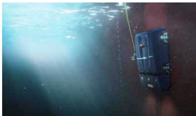
Jotun HullSkater working underwater, Semcon
